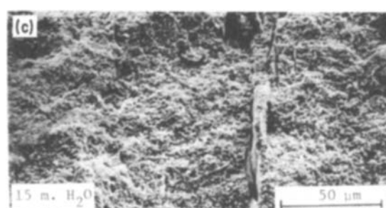
Figure 8 Fracture surface scanning electron micrograph of sintered ZrO_2 samples formed by hydrolytic condensation of Zr(OC_4H_9)_4 with different amounts of water in n-butyl alcohol at 5% wt equivalent ZrO_2 concentration. (There was no consolidation in the 1 mol hydrolysed sample shown in Fig. 8a during sintering.)
